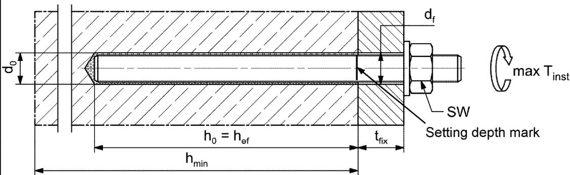
**Commercial standard threaded rods, washers and hexagon nuts may also be used if the following requirements are fulfilled**
