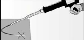
Extrude approximately 10 cm of material out until the resin is evenly grey in colour. Do not use mortar that is not uniformly grey |
